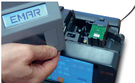
TWN4 MultiTech Mini Reader inside of "EMAR 205" cash register with the option of handling electronic RFID tickets.
