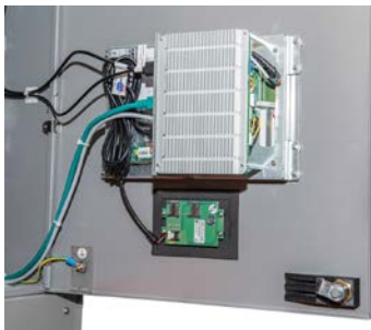
Elatec's TWN4 MultiTech 2 BLE card reader, integrated in the myRENZbox ( briefkasten.de ).
