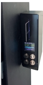
Apollo Games USB-based hardware is attached to the side of cabinet. For user interaction: buttons, a LCD screen and TWN4 Smartcard are implemented.
